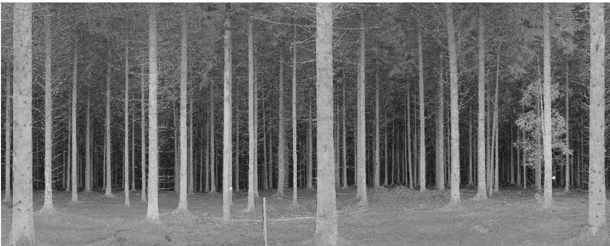
Figure 3: Intensity image derived from terrestrial laser scanning data.
