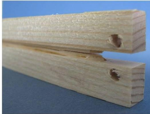
Figure 8a. Modified DCB specimen in RL crack configuration of wood.
