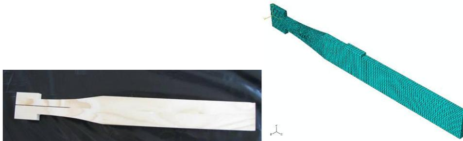
Figure 6. Photograph of the PTENF-specimen and meshed 3D (ABAQUS) model of the geometry
