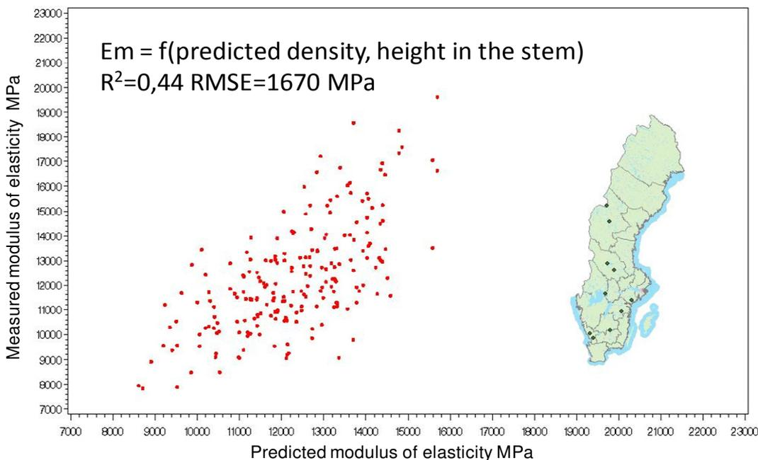
**Figure 5.** Predicted vs. measured modulus of elasticity (MOE) of spruce boards based on the new model developed with contribution from Woodvalue (Hannrup & Wilhelmsson, manuscript). Model developed from sample trees of the Swedish spruce stem bank (Luleå Tech University, Chalmers and SLU). Experiments located according to map.
