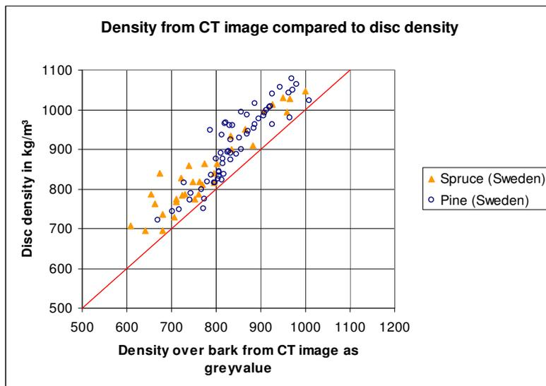
**Figure 7.** Variation of mean log wood density measured by CT scanning and on top disc of logs
