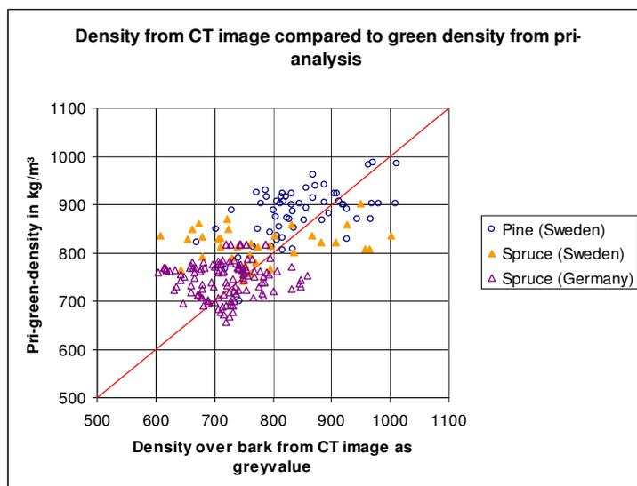
**Figure 6.** Variation of mean log wood density measured by CT scanning and predicted by pri-simulation.
